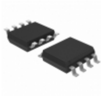
AT24C512C-SSHM-T Microchip Technology IC EEPROM 512KBIT 1MHZ 8SOIC
