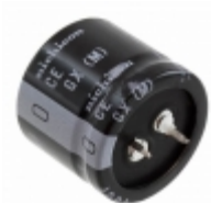
LGX2E471MELB25 Nichicon CAP ALUM 470UF 20% 250V SNAP
