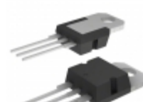
MIC29500-5.0BT Microchip Technology IC REG LDO 5V 5A TO220-3
