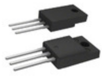
ACST1635-8FP STMicroelectronics TRIAC 800V 16A TO220FPAB
