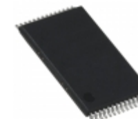
AS7C256B-12TINTR Alliance Memory, Inc. IC SRAM 256KBIT 12NS 28TSOP
