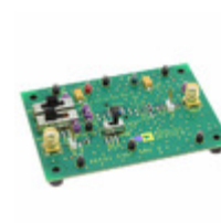
AD603-EVALZ ADI (Analog Devices, Inc.) BOARD EVALUATION FOR AD603
