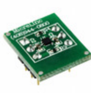
MIC94325YMT-EV Micrel / Microchip Technology EVAL BRD ADJ 500MA LDO MIC94325
