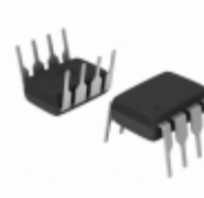
TC429CPA Micrel / Microchip Technology IC MOSFET DRIVER 6A HS 8DIP
