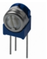
3329X-1-101 Bourns, Inc. TRIMMER 100 OHM 0.5W PC PIN SIDE
