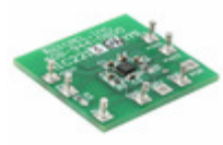
MIC2213-GNYML-EV Micrel / Microchip Technology EVAL BOARD ADJ SEQ POWER
