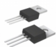
IXFP8N50PM IXYS MOSFET N-CH 500V 4.4A TO-220
