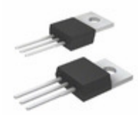
IXFP90N20X3 IXYS Corporation 200V/90A ULTRA JUNCTION X3-CLASS
