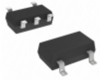
AN80L48RMS Panasonic Electronic Components IC REG LDO 4.8V 0.15A MINI5D
