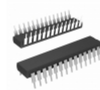
U62256ADK07LLG1 Alliance Memory, Inc. IC SRAM 256KBIT 70NS 28DIP
