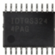
QS3244PAG8 IDT, Integrated Device Technology Inc IC BUS SWITCH 16:8 20-TSSOP
