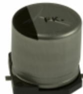
EEE-FK0J152P Panasonic Electronic Components CAP ALUM 1500UF 20% 6.3V SMD
