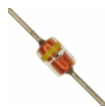
MTZJT-774.3A Rohm Semiconductor DIODE ZENER 4.3V 500MW MSD
