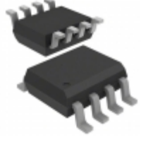
AD8215YRZ-R7 Analog Devices Inc. IC CURRENT MONITOR 0.15% 8SOIC
