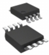
MCP4802T-E/MS Microchip Technology DAC 8BIT DUAL SPI/VREF 8MSOP
