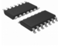
BTS5236-2EKA International Rectifier (Infineon Technologies) IC SWITCH PWR HISIDE DSO-14
