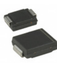
SM15T27AY STMicroelectronics TVS DIODE 23.1VWM 48.3VC SMC
