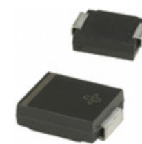
SM15T27AHE3/9AT Vishay Semiconductor Diodes Division TVS DIODE 23.1VWM 37.5VC SMC
