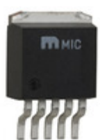
MIC29372BU Microchip Technology IC REG LDO ADJ 0.75A TO263-5
