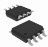
IRF7807APBF Infineon Technologies MOSFET N-CH 30V 8.3A 8-SOIC
