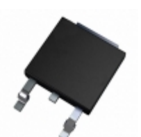
IXTY1N80P IXYS MOSFET N-CH 800V 1A TO-252
