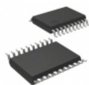
MCP4351-502E/ST Microchip Technology IC POT 8BIT QUAD 5K 20TSSOP
