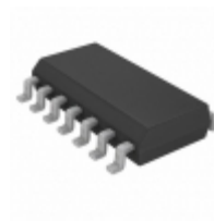
PIC16LF1574-I/SL Microchip Technology IC MCU 8BIT 7KB FLASH 14SOIC
