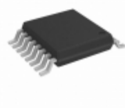
PI6C10806LE Diodes Incorporated IC CLK BUFFER 1:6 250MHZ 16TSSOP
