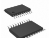
PI6C10807LE Diodes Incorporated IC CLK BUF 1:10 250MHZ 20TSSOP
