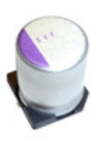
25SVF56M Panasonic CAP ALUM POLY 56UF 20% 25V SMD
