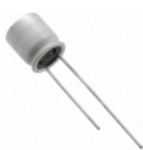
100SXE15MX Panasonic CAP ALUM POLY 15UF 20% 100V T/H
