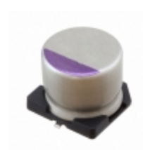
100SXV18M Panasonic CAP ALUM POLY 18UF 20% 100V SMD
