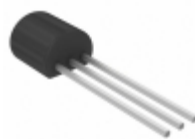
2SA0720ARA Panasonic Electronic Components TRANS PNP 70V 0.5A TO-92
