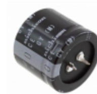
LGY1J472MELC30 Nichicon CAP ALUM 4700UF 20% 63V SNAP
