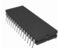
AD7874AQ ADI (Analog Devices, Inc.) IC DAS 12BIT 4CH 5V 28-CDIP
