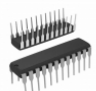
AD7228ABNZ Analog Devices Inc. IC DAC 8BIT OCTAL W/AMP 24-DIP
