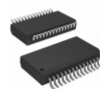
PIC32MM0032GPL028-E/SS Micrel / Microchip Technology 32KB FLASH, 8KB RAM, 79 COREMARK
