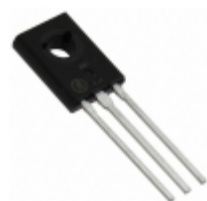
BD442G ON Semiconductor TRANS PNP 80V 4A TO-225AA
