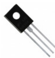
BD442STU AMI Semiconductor / ON Semiconductor TRANS PNP 80V 4A TO-126
