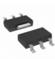
BD450M2FP3-CE2 Rohm Semiconductor IC REG LDO 5V 0.2A SOT-223-4
