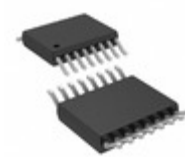
LTC2327IMS-18#PBF ADI (Analog Devices, Inc.) IC ADC 18BIT 500KSPS 16MSOP
