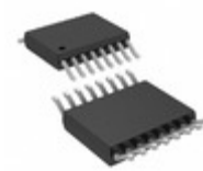
LTC2328CMS-18#PBF ADI (Analog Devices, Inc.) IC ADC 18BIT 1MSPS 16MSOP
