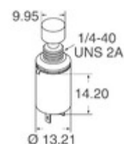
MSPM101B0 TE Connectivity ALCOSWITCH Switches SWITCH PUSH SPST-NC 0.1A 50V
