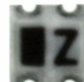
EHF-FD1513 Panasonic Electronic Components POWER DIVIDER 1720-1790MHZ
