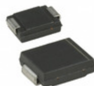
SM30T30CAY STMicroelectronics TVS DIODE 26VWM 42.1VC SMC
