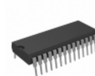
AT28C64B-15PC Microchip Technology IC EEPROM 64KBIT 150NS 28DIP
