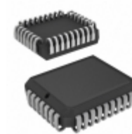
AT28C64B-15JU-235 Microchip Technology IC EEPROM 64KBIT 150NS 32PLCC
