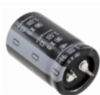
LGX2W221MELA40 Nichicon CAP ALUM 220UF 20% 450V SNAP
