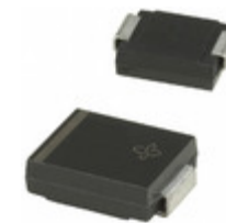
SS34HE3_A/I Electro-Films (EFI) / Vishay DIODE SCHOTTKY 40V 3A DO214AB
