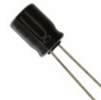
EEU-EB1A471B Panasonic Electronic Components CAP ALUM 470UF 20% 10V RADIAL
