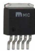
MIC59300-1.2WU Microchip Technology IC REG LDO 1.2V 3A TO263-5
