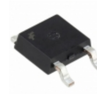
FQD5N15TM Fairchild/ON Semiconductor MOSFET N-CH 150V 4.3A DPAK
