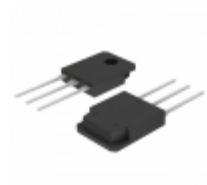
IXFH20N85X IXYS 850V/20A ULTRA JUNCTION X-CLASS
