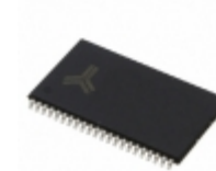
AS7C31026B-12TCN Alliance Memory, Inc. IC SRAM 1MBIT 12NS 44TSOP
