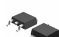
RD3P130SPTL1 LAPIS Semiconductor PCH -100V -13A POWER MOSFET
