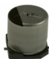
EEE-FK1H221P Panasonic Electronic Components CAP ALUM 220UF 20% 50V SMD
