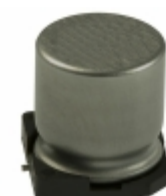
EEE-FK1H331AQ Panasonic Electronic Components CAP ALUM 330UF 20% 50V SMD
