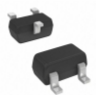
BC857BT-7-F Diodes Incorporated TRANS PNP 45V 0.1A SOT523
