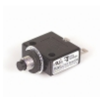
CLB-133-11-B-3-A-B-A Carling Technologies CIR BRKR THRM 13A 250VAC 32VDC
