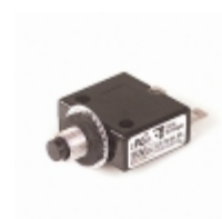
CLB-053-11-B-3-A-B-A Carling Technologies CIR BRKR THRM 5A 250VAC 32VDC
